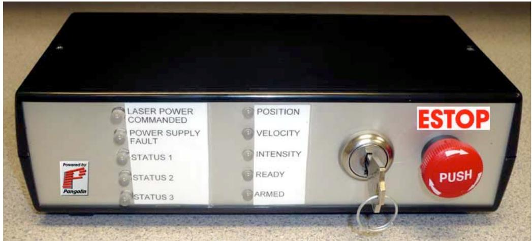
PASS may be controlled by, and may illuminate LEDs on an external control panel that is connected to PASS. Below is a description of the control panel connections. When PASS is not connected to an external control panel, then PASS will automatically reset into a “ready” state shortly after power up. When PASS is connected to an external control panel, then PASS will not power up in a “ready” state and instead, will wait for the “Manual Reset” from the control panel.
