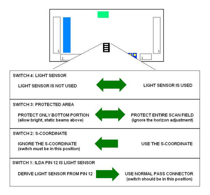
With the PASS board in this orientation, Switch 4 is at the top. When this switch is moved to the left (on), the light sensor input is ignored. You would move the switch to this position if you are not using a light sensor. When this switch is moved to the right (off), the light sensor input is monitored, and an additional level of safety is provided. Pangolin ships the PASS board with this switch turned on.
