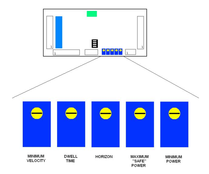
PASS includes a number of adjustments and switches that can be used to customize operation to a particular projector or projection scenario. Below you will see the PASS board and location of five adjustment potentiometers. The operation of each potentiometer is described below.
